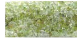
Grade 1 equivalent to 16/30 Grade sand
