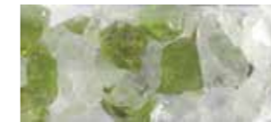
Grade 3 equivalent to 6mm gravel
