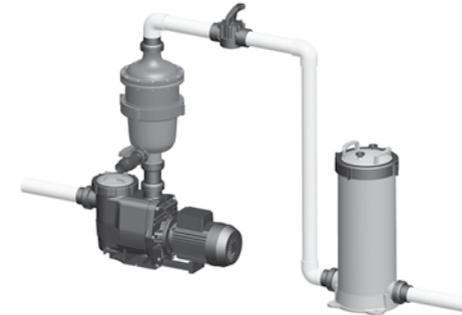
Installation with 2 way shut off valve
