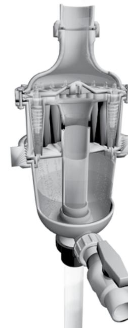
Incoming water is guided by a diverter plate so that it enters multiple hydro cyclones tangentially generating a strong centrifugal effect. This spins the sediment out to the hydro cyclone's wall and then spirals it down to the sediment chamber, while the cleansed water spirals upwards.
